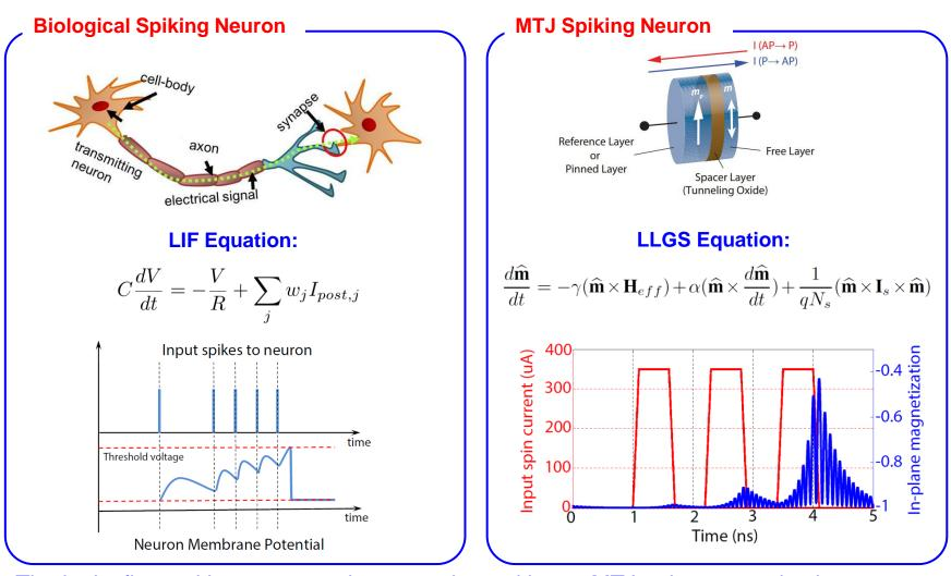
The leaky fire and integrate can be approximated by an MTJ – the magnetization dynamics mimics the leaky fire and integrate operation
